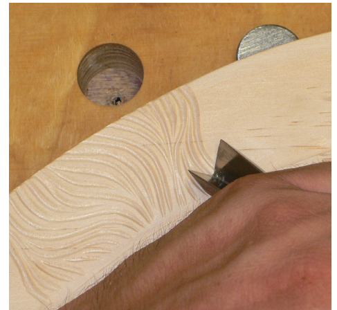
Photo 11: Random V-grooves with tool #8
